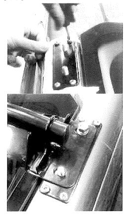
8. Mount the visor on the main bracket according to the drawing.
