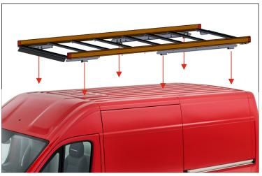
**STEP-2** Match the brackets with the factory plugs on the vehicle.
