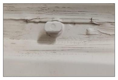
**STEP-1** Brackets need to be located to this factory plug on the vehicle.
