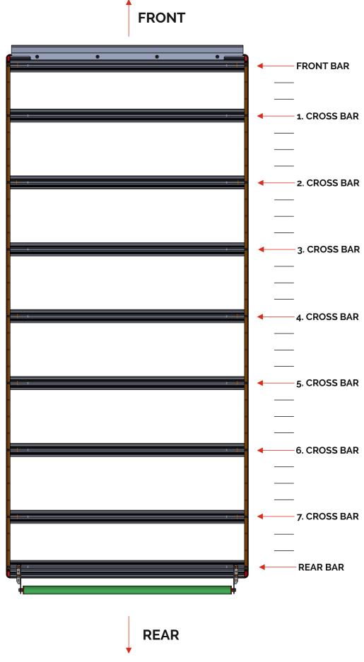
CROSS PROFILES WILL BE MOUNTED AS SHOWN ON FIGURE ABOVE.
