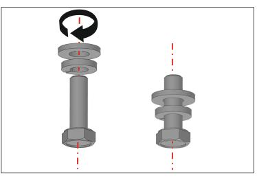
**STEP-4** Attach spring washer first then flat washer to M6x25 hex bolts
