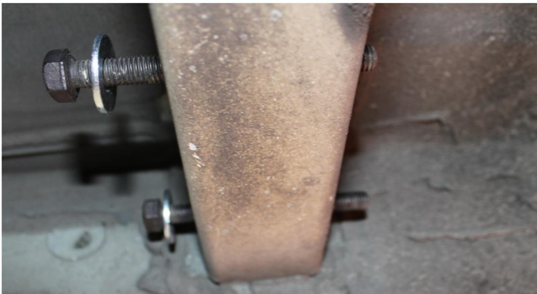
**Place the mounting brackets left and right on the bolts and mount the washers and nuts on it**
