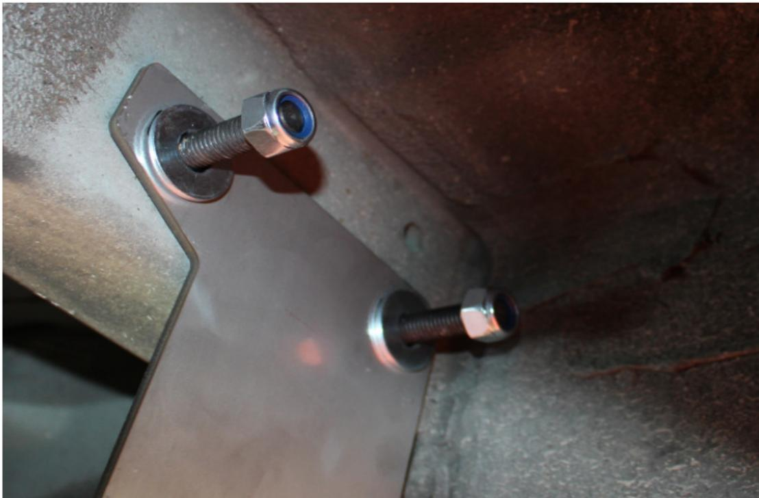
**Place the step on the brackets and tighten the nuts by hand**
