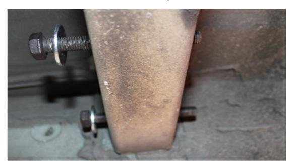
Place the mounting backets left and right on the bolds and mount the washers and nuts on it NOTE , DO NOT TIGHTEN YET
