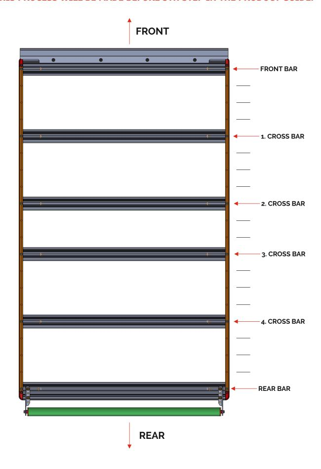
CROSS PROFILES WILL BE MOUNTED AS SHOWN ON FIGURE ABOVE.
