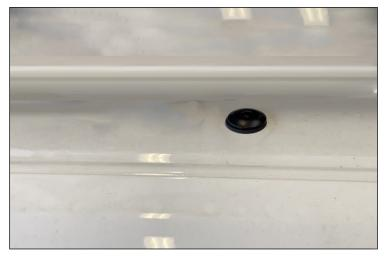
**STEP-1** Remove factory rubber plugs as shown.
