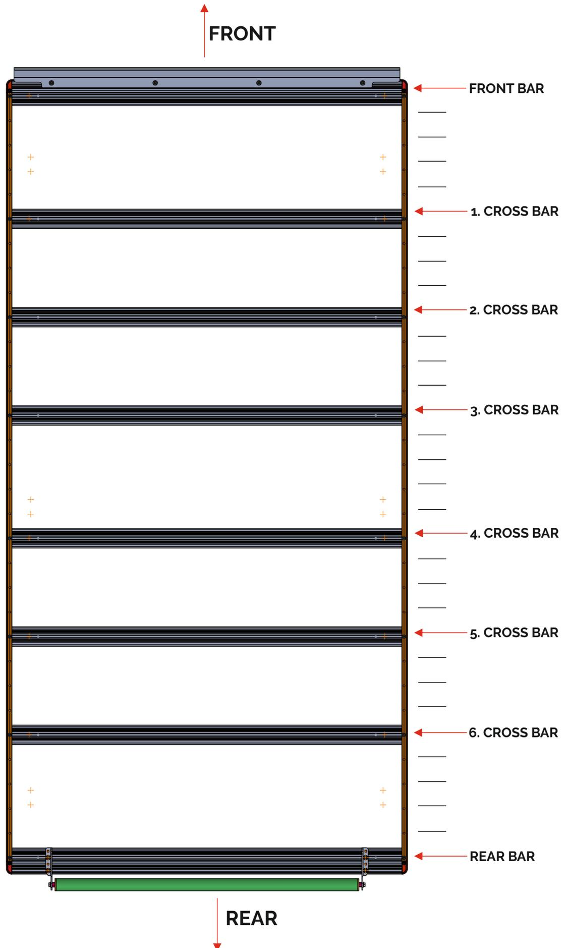
**CROSS PROFILES WILL BE MOUNTED AS SHOWN ON FIGURE ABOVE.**
