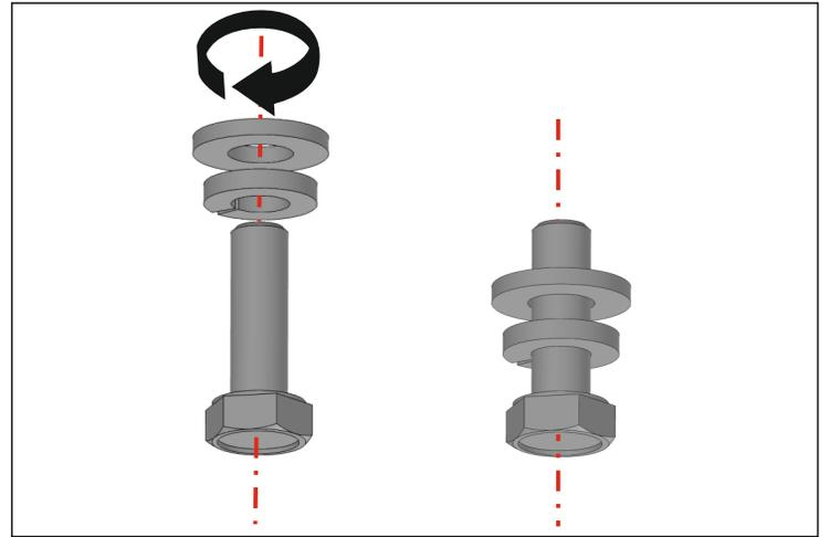
**STEP-4** Attach spring washer first then flat washer to M8x25 hex bolts
