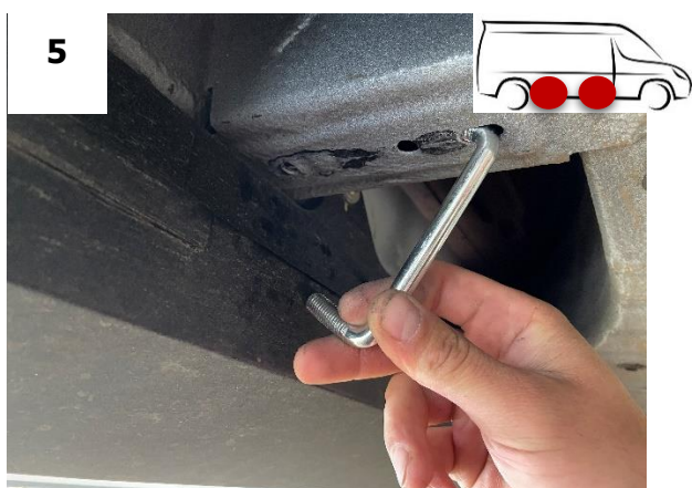
U bolt is connected as shown.
