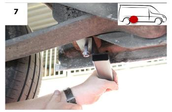
Fix the passenger front bracket to the vehicle with the help of M10 nut.
