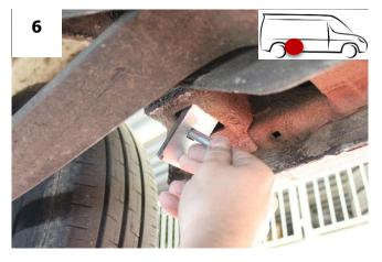
To mount the passenger front bracket, insert the HTCOR3 + M10x25 hex bolt into the area marked in the figure.
