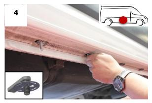
Insert the HTC 230 bolt into the holes and secure it with the HTC 269 clip.
