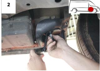
To mount the passenger front bracket, insert the HTCOR6 + M10x45 square neck bolt into the area marked in the figure.
