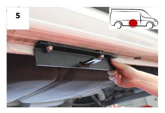
Fix the passenger center bracket to the vehicle with the help of M10 nut.
