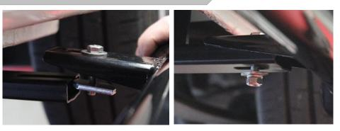
Important! After positioning the step in the appropriate position, tighten the M8 nuts with 25 Nm and the M10 nuts with 50 Nm.
