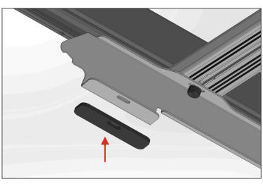
**STEP-2** Put supplied rubber part in the bottom part of the bracket on the vehicle.
