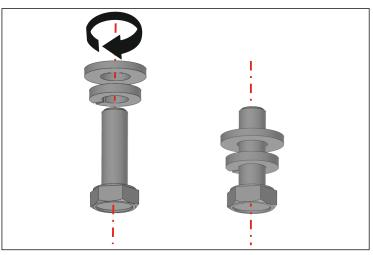
**STEP-4** Attach spring washer first then flat washer to M8x25 hex bolts
