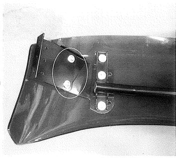
3. Place the side bracket on the A-pilar 655mm from the bottom line of the door pilar and mark the hole positions (remember to mark all mounting holes of the sidebracket).
