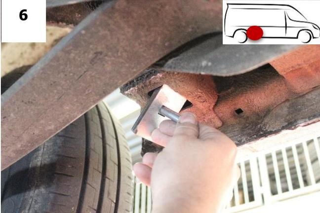
To mount the passenger front bracket, insert the HTCOR3 + M10x25 hex bolt into the area marked in the figure.
