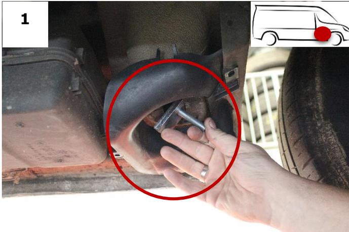
To mount the passenger front bracket, insert the HTCOR6 + M10x45 square neck bolt into the area marked in the figure.
