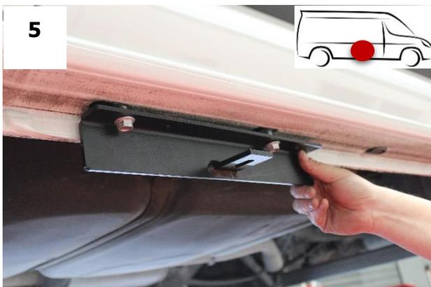
Fix the passenger center bracket to the vehicle with the help of M10 nut.
