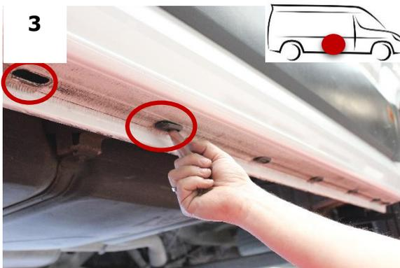
Remove the gaskets marked in the figure in order to mount the passenger center bracket.
