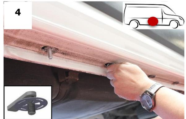
Insert the HTC 230 bolt into the holes and secure it with the HTC 269 clip.
