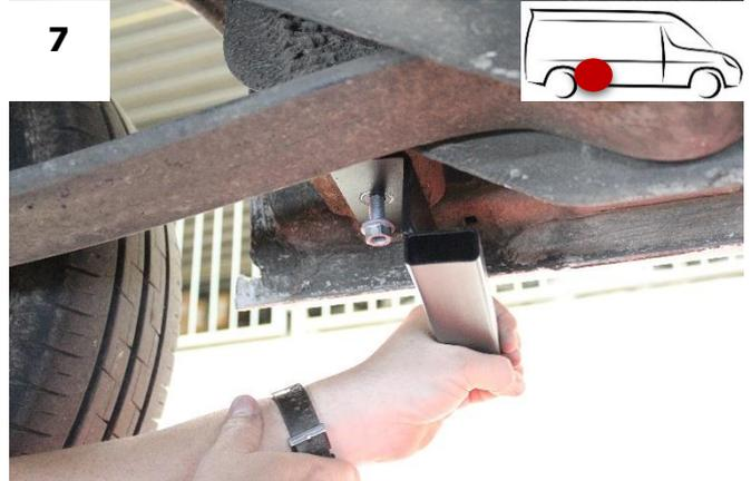
Fix the passenger front bracket to the vehicle with the help of M10 nut.
