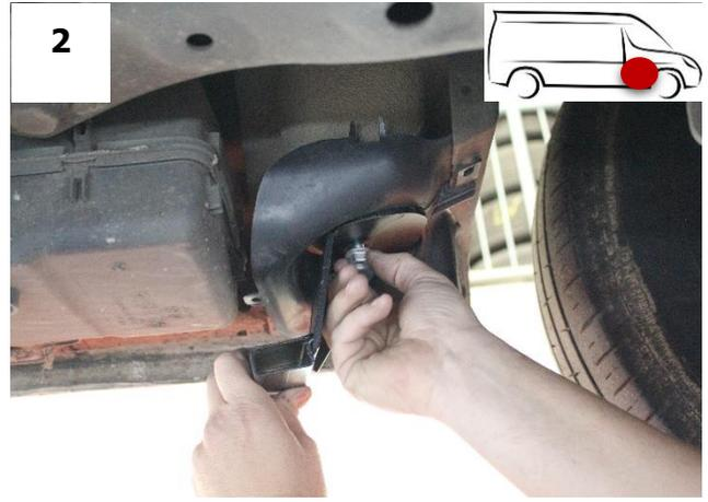
Fix the passenger front bracket to the vehicle with the help of M10 nut.
