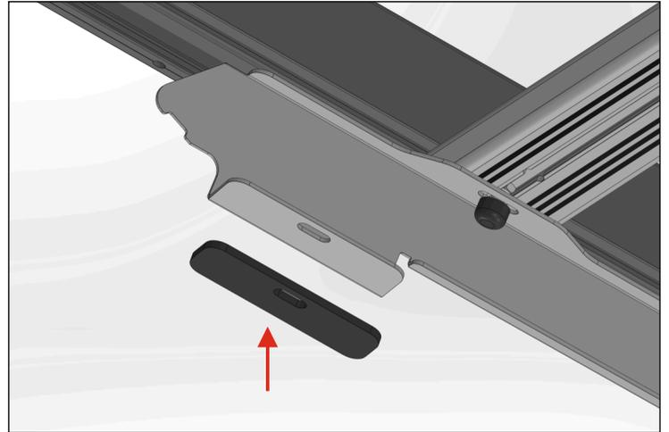
**STEP-2** Put supplied rubber part in the bottom part of the bracket on the vehicle.
