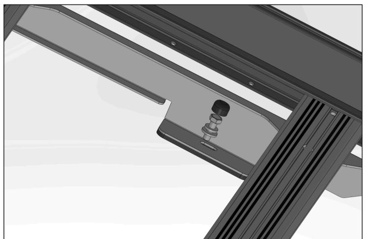
**STEP-6** Fix the bracket with bolt to the holes on the vehicle. Repeat this process for all brackets.
