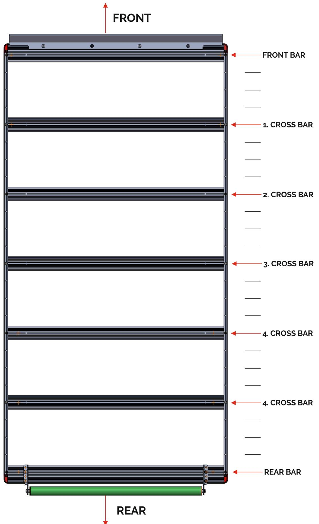
**CROSS PROFILES WILL BE MOUNTED TO 4TH HOLE AFTER EVERY 3 HOLES AS SHOWN ON FIGURE ABOVE.**
